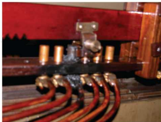
Figure 4: Arcing at OLTC contacts
